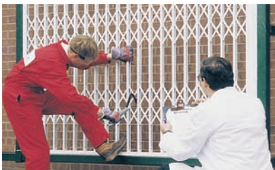
SeceuroGuard 1001 undergoing a simulated attack test
